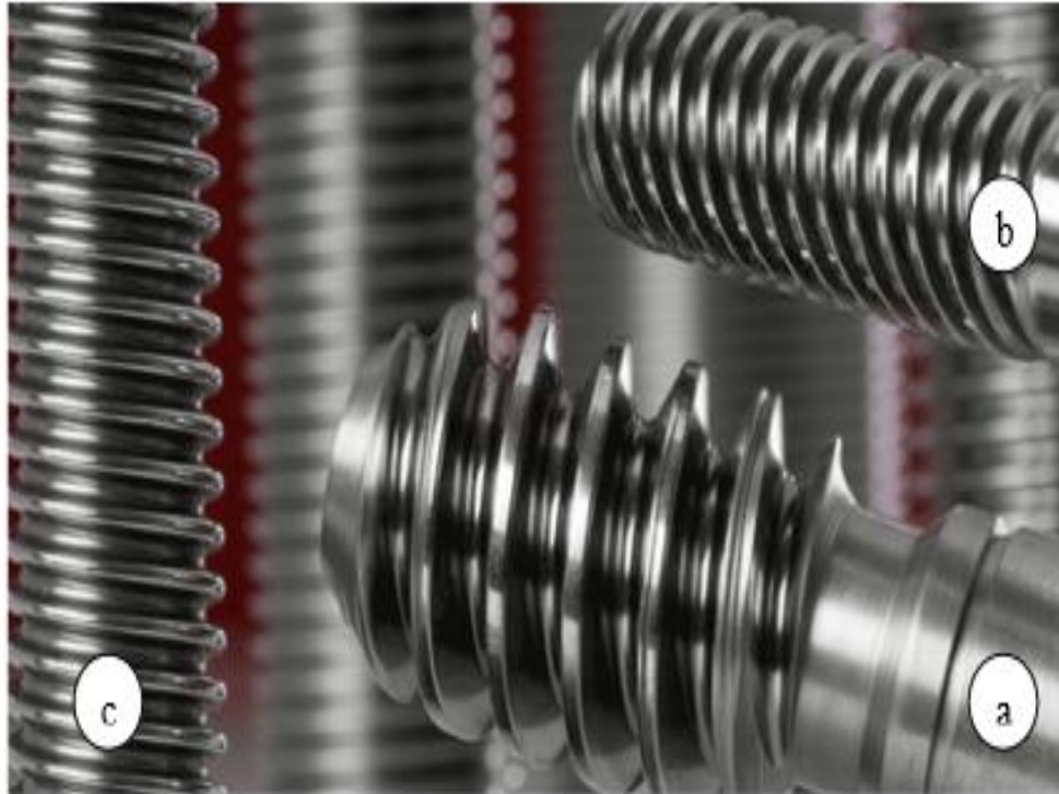
Fgi.12.1.2.Filete(a-trapezoidal; b-pătrat; c-rotund)
